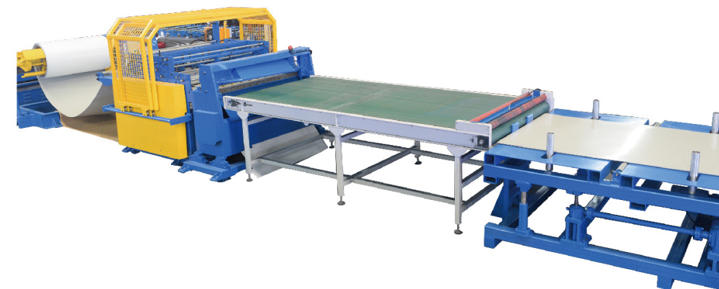
△ 卷边机, 宽度可调 Hemming Machine Width Variable
